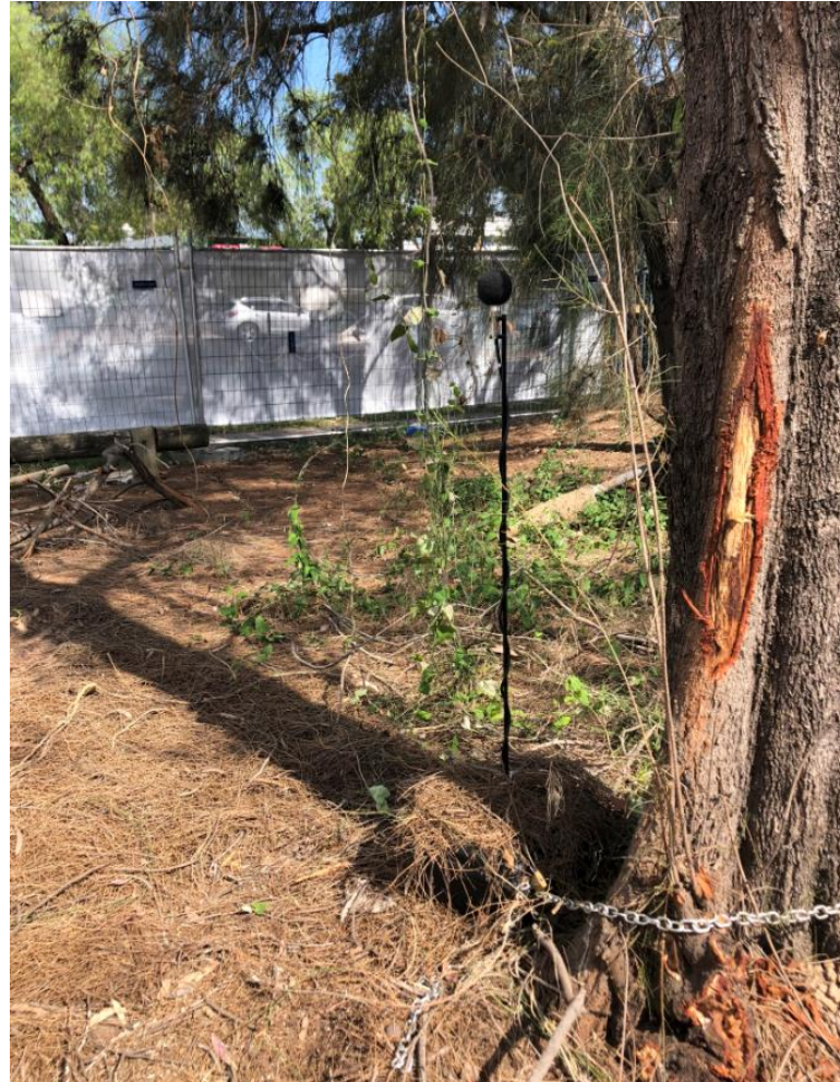
Figure 4: Unattended Noise Monitor Installed on the stage 1 project site
